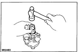
(b) Using a socket wrench and hammer, drive in a new oil seal.
