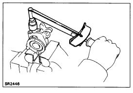
(c) Install and torque the pressure port union.
