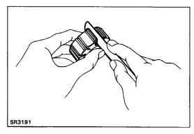
(b) Using a feeler gauge, measure the clearance between the rotor groove and vane plate.
