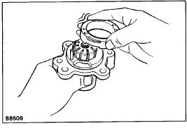
6. REMOVE CAM RING, ROTOR AND VANE PLATES NOTICE: Be careful not to scratch the cam ring, rotor or vane plates.
