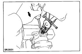
(e) Using snap ring pliers, install the snap ring.
