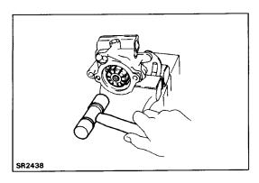
(c) Align the hole of the front plate and straight pin and tap in the pump shaft with a plastic hammer.NOTICE: Be careful not to damage the oil seal and 0-rings.
