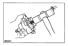
(d) Using a plastic hammer, lightly tap the rotor shaft out of the front housing.
