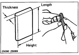
HINT: There are five vane lengths with the following rotor and cam ring numbers:
