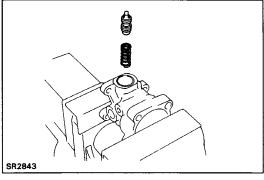
(c) Remove the flow control valve and spring.
