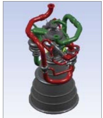
Rendering of the Integrated Powerhead Demonstrator shows its innovative plumbing for routing fuel and oxidizer to the combustion chamber.
