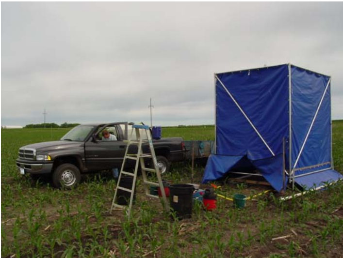
Figure 8. Rainfall simulator centered over top of microplot area. Rainfall nozzle was placed at >3 m above plot surface to approximate terminal rainfall velocity.
