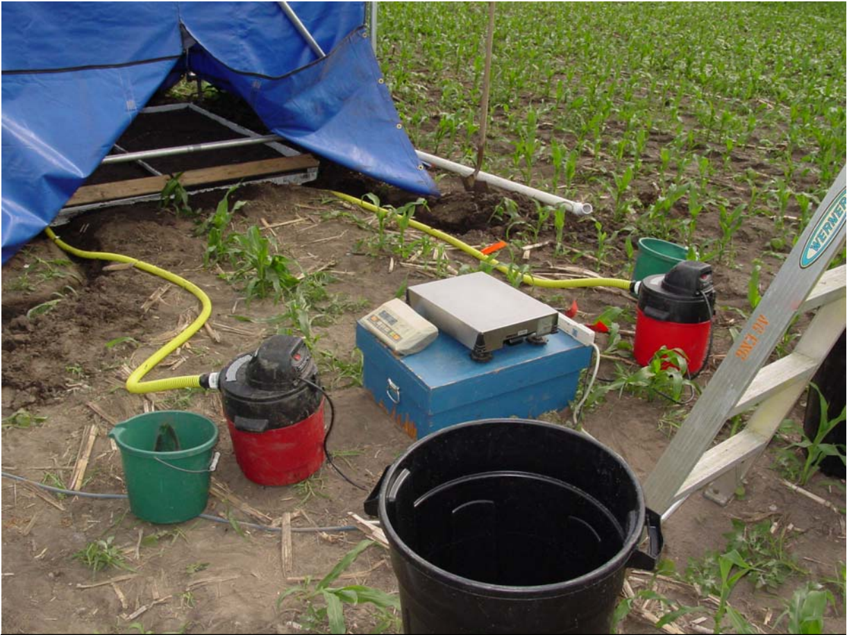
Figure 9. Surface runoff was collected at 5 min intervals, weighed, and placed into a composite sampling container. Composite samples were collected at the end of 30 minutes and analyzed for TDP and TP concentrations.
