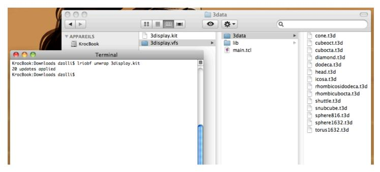
All data from starkit's virtual file system are extracted to 3display.vfs directory. The only required script is main.tcl at root wich is automatically sourced when a starkit is run. The two first lines of main.tcl should be:
