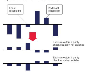
It should be noted that a parity-check equation relates a set of scattered bits by parity. The bit-to-check step can be viewed as an information-gathering function. One piece of information gathered is whether or not the parity-check equation is satisfied, and the sign of each LLR bit is used
