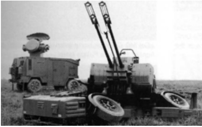
The Skyguard and 35 mm gun. The Skyguard has a search radar range of 25 km and uses a tracking radar to carry out engagements. Each Skyguard is normally connected to two 35 mm guns (which can be up to 500 m away) that are remotely controlled from within the Skyguard itself. The guns fire 1,100 rounds per minute and can be used against all types of aircraft plus cruise missiles. (DND Photo)
