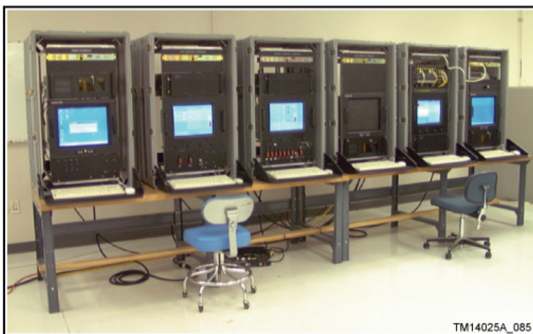
Figure 2-5. Minotaur I Launch Control Consoles Configuration
