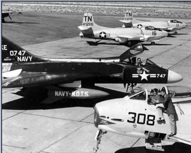
NOTS Project (“NOTSNIK”) test shape ready for flight on F4D, Armitage Field, 1958.
