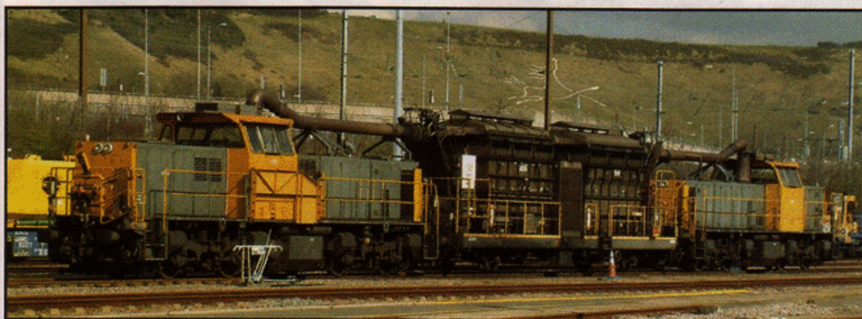
Two of the maintenance locomotives, each with its own 50 ton scrubber wagon are shown here in their old configuration. These 1.2 MW locomotives were manufactured by Krupp in the early '90s with MTU 12V396C13 diesel engines, using the best technology available at that time.
