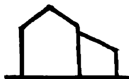
Lean-to roof at shallower pitch and stepped.
