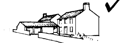
House set well back. Side entry double garage and turning area. Staggered garage plan with neighbour.
