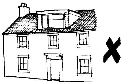
Large flat-roofed dormer dominates elevation.
