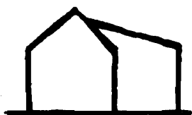
Lean-to roof too shallow. Poor junction with main roof.
