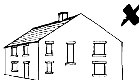
Square plan form gives over-wide gable. Effect worsened by having too many openings.
