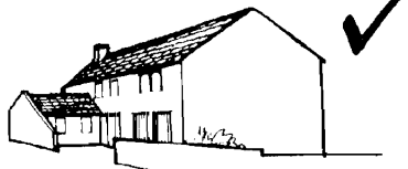
Wider frontage detached house with integral double garage. Note accommodation wing can be brought almost to back of footway.
