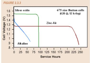
A comparison of discharge profiles of primary battery systems
