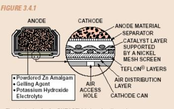
The electrodes for the DURACELL® zinc air cell are shown.
