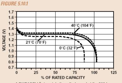
A DURACELL<sup>®</sup> zinc air battery discharged at the 300 hour rate at 0°C (32°F), 21°C (70°F), and 40°C (104°F).
