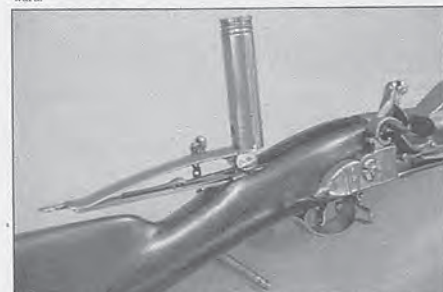
Figure 5-Further movement of the breech cover causes the chamber piece to pop up vertically for loading.
