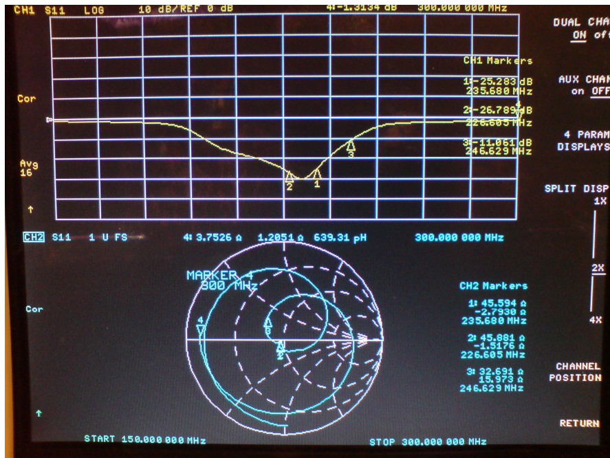
Figure 8.1.5: Reflection coefficient s_{11} vs. frequency for a Renkwitz Yagi covered by an approx. 2.5 mm thick ice layer, applied by repeatedly spraying water onto the antenna elements with a spray bottle. For this measurement the antenna was kept at an ambient temperature of -15^{\circ}\text{C} . The -20\text{ dB } s_{11} pass-band has now shifted to approx. (216 – 239) MHz and no longer meets the (235 \pm 6) MHz band-width requirement on the high-frequency side.
