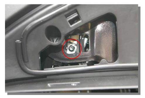
In the photo below you can see both (silvery) screws which clamp the window to the mechanisms.
