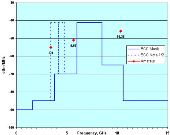
The plot above is the mask level specified in the Annex of the Draft Decision, compared to the protection levels that ECC Report 64 [5] determined are necessary for the Amateur Services. Note that 3.1-3.4GHz may also be investigated according to the draft decision.
