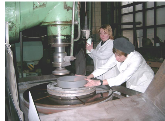
Preparation of cylindrical surface and end surface with accuracy 0.1 mm
