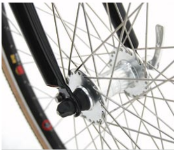
Tough, large flange, Shimano XT 48 hole tandem hubs handbuilt in to bomb proof Sun Rhino rims.
