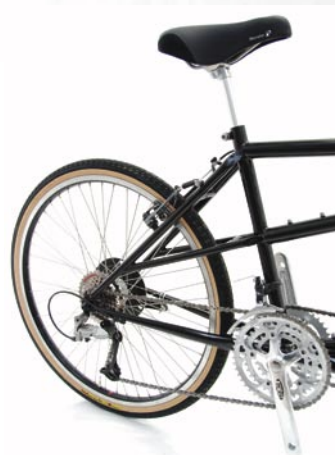
Double marathon frame design for increased strength and stiffness and stability.
