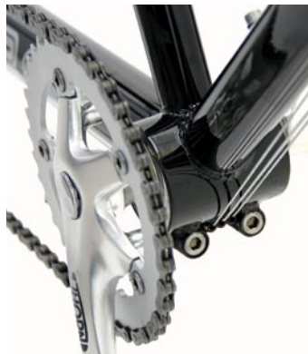
Quick, simple and reliable eccentric bottom bracket chain adjustment.
