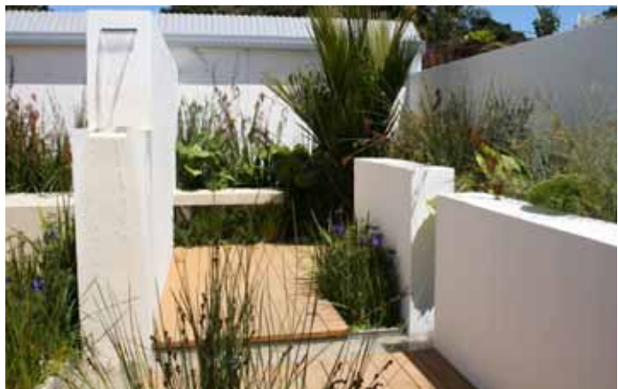
Figure 41: A vertical water tank separates areas in an outdoor residential courtyard and the overflow spills as a water feature into several raingardens. Designers: Douglas, Kirsten Sach and Zoe Carafice, Unitech, for Ellerslie International Flower Show, Auckland, 2007. Photo: Maria Ignatieva
