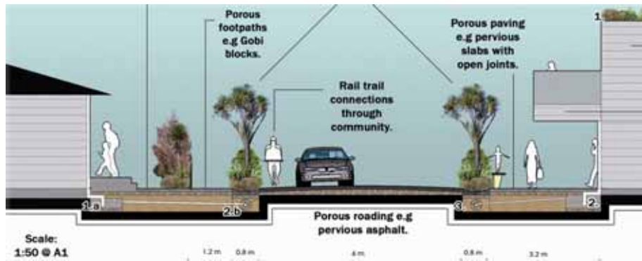
Figure 13: Cross section of narrow street for proposed new Liffey Spring Subdivision in Lincoln Village, South island, New Zealand. Design: Simon Moultrie, 2007
