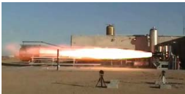
AirLaunch has completed 34 test fires of the second stage engine on the Horizontal Test Stand (HTS)
