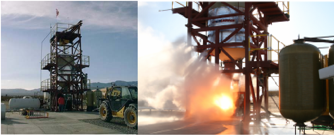
QuickReach™ Test Fires of IS2 in VTS, including longest VaPak burn in history (191 seconds)
