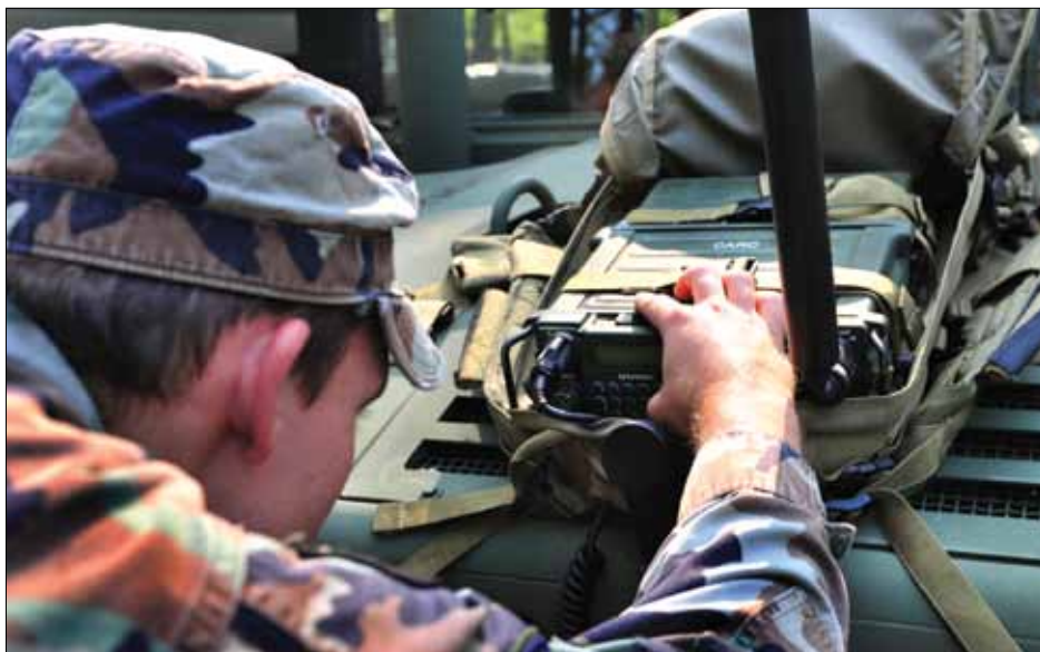
An Air Force and tactical air control party practice using a PRC-117F (primary man-portable radio) during a TACP exercise. The TACP members are specialists who are assigned to combat units. They advise ground forces on aircraft employment and capabilities, coordinate and control aerospace operation and participate in battle planning. (U.S. Air Force photo/Airman 1st Class Amber E. N. Jacobs)
