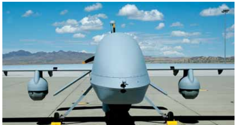
Gray Eagle unmanned aircraft with TRICLOPS payload configuration. [Photo courtesy of U.S. Army]
