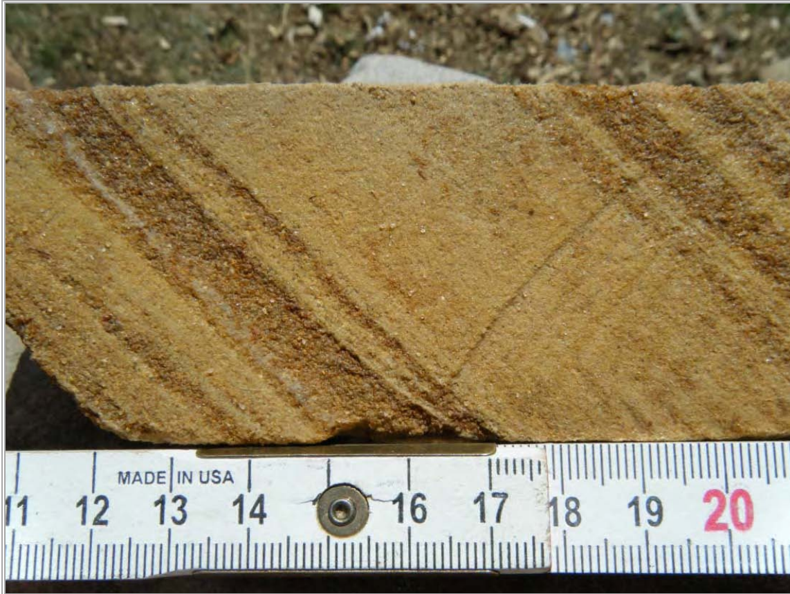
Figure 14-1 Typical Porosity at Limosna LMD048 @ 468.30 m
