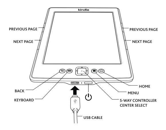
To charge your Kindle, connect it to the USB cable. Then connect the opposite end of the USB cable to a computer or power adapter (sold separately).
