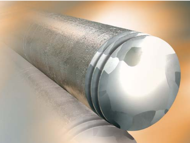
Nb RRR ingot with defined coarse-grain structure
