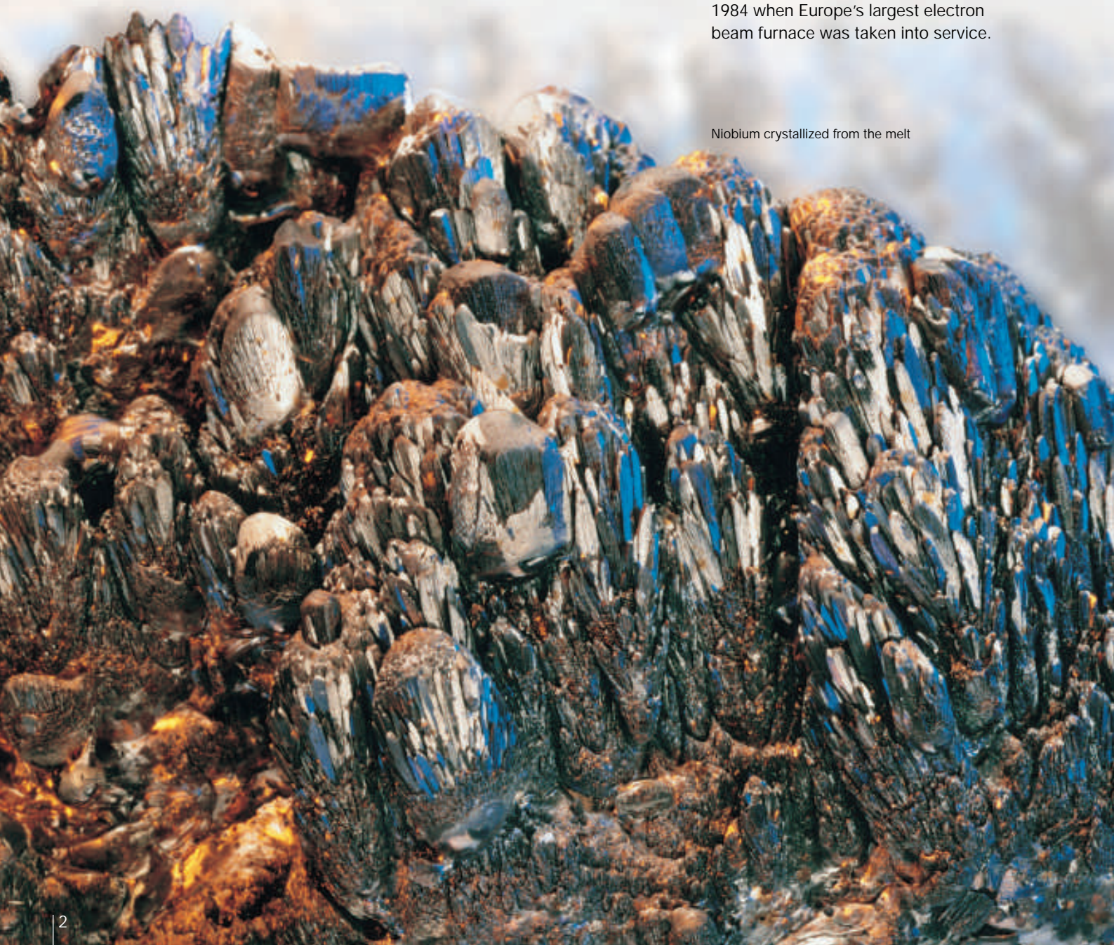
Melting niobium under high vacuum in the electron beam furnace at a temperature of approx. 2600°C
