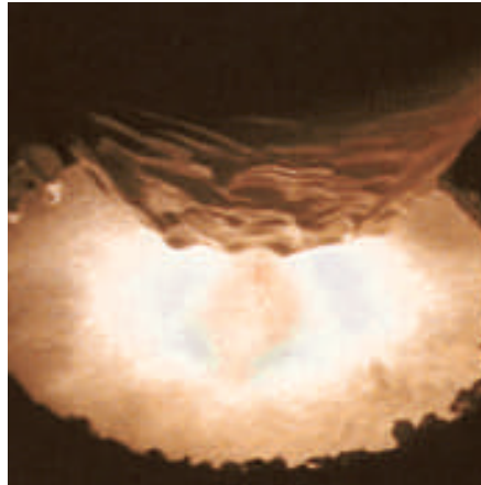
Melting niobium under high vacuum in the electron beam furnace at a temperature of approx. 2600°C
