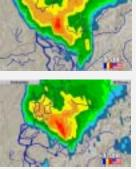
Reflectivity as measured by the ANM radar for  $0.5^{\circ}$  antena elevation angle, 12 August 2002, 1700 UTC (top) and 1710 UTC (bottom) respectively few minutes after Facaeni village was struck
