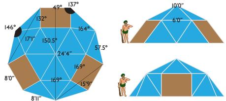
For the second (the **Quad-dome**) four standard roofs are made and leant together around a square. The remaining holes are filled, with a square on top and four squares cut accross the middle round the side. The diagonally cut squares are vertical:
