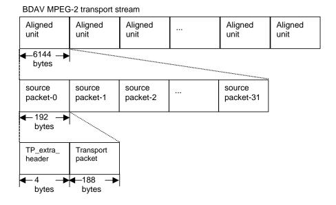
Figure 4-1 – Structure of BDAV MPEG-2 transport stream
