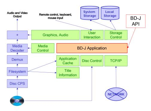
Figure 7-4 Interfaces between a BD-J application and BD-J System software
