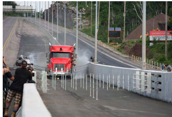
Test truck using the runaway ramp
