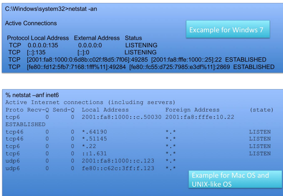
Figure 9 : Verifying communication status with a netstat command
