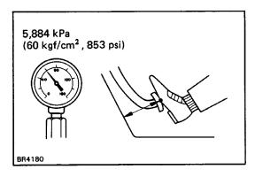
(d) With the engine running, hold the brake pedal depressed for about 1 0 seconds with the pressure at 5,844 kPa (60 kgf/cm<sup>2</sup>, 853 psi), and check that there is no change in the pedal reserve distance. If there is a change in the brake pedal reserve distance, inspect the brake actuator.
