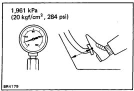
(c) With the engine off, hold the brake pedal depressed for about 10 seconds with the pressure at 1,961 kPa (20 kgf/crn², 284 psi), and check that there is no change in the pedal reserve distance. If there is a change in the brake pedal reserve distance, check the brake line, master cylinder and wheel cylinder for fluid leakage.
