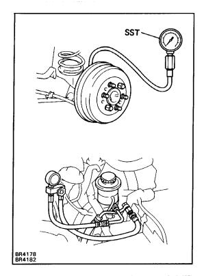
With the engine running, the brake and power steering fluid pressure should conform to the following table.
