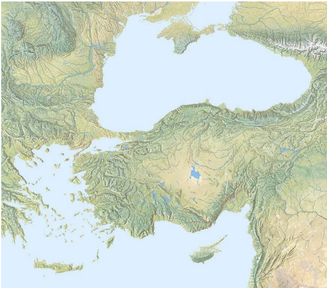
Figure 1. A portion of Hal Shelton's 1:5,000,000-scale New Europe map painted ca. 1968. The original measures 107 x 137 centimeters. Drainages and water bodies are photomechanical additions to the original art. Courtesy of Rand McNally & Company.
