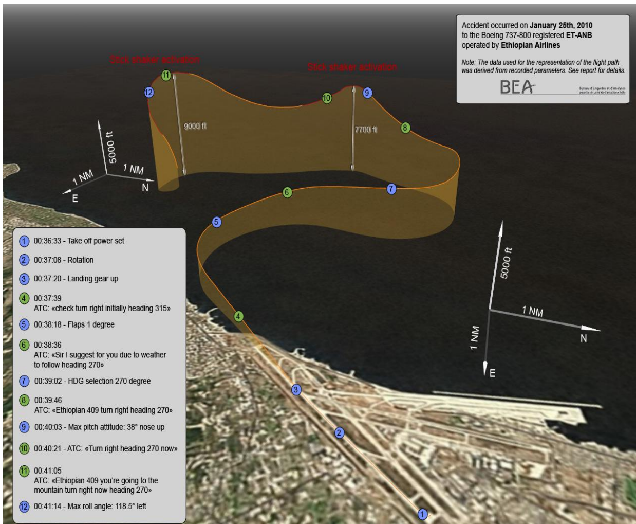
Figure 12: ET 409 Flight 3 D profile
