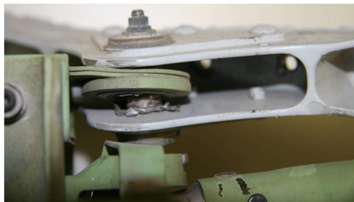
Figure 17: Left Inner Attachment Bearing
