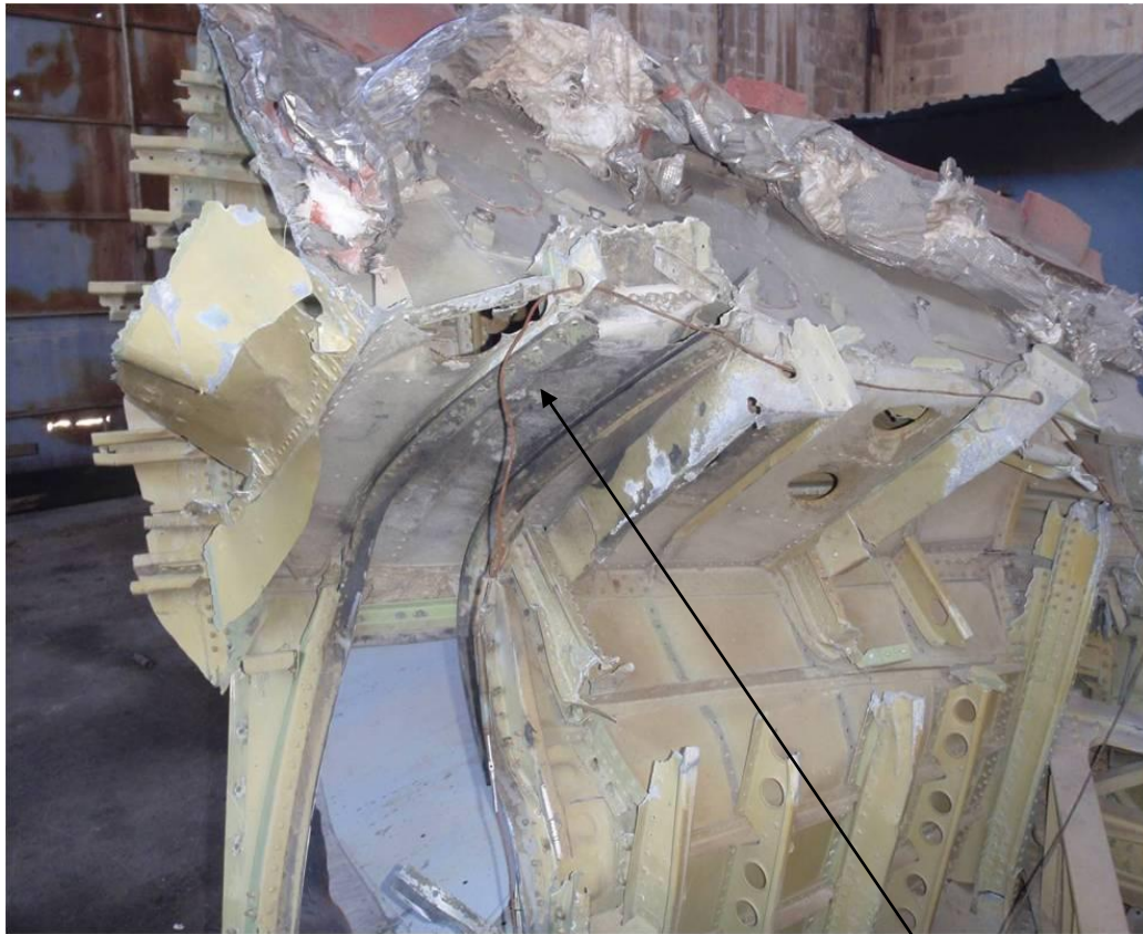
Figure 14: The APU Exhaust area showing the Black Soot
