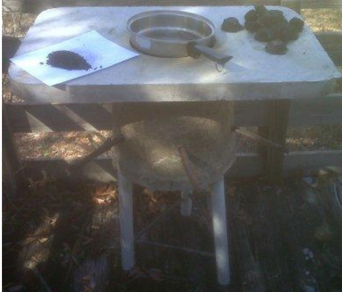
Kenaf Stove w/ tabletop, displaying bio-char on L and molded charcoal briquettes on R. Sticks and cooking pot are used to cut- off air flow and induce bio-char production.
