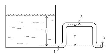
A very large reservoir is filled to a height H above a discharge outlet which sends water through a vertical loop before discharging it at point (3) into the atmosphere. Water weighs 62.4 lbf per cubic foot. At point (1), the pipe has a cross-sectional area  $A_1 = 1.00 \, ft^2$ , at point (2)  $A_2 = 1.00 \, ft^2$ , while at (3),  $A_3 = 0.75 \, ft^2$ .  $H = 1.00 \times 10^3 \, ft$  and
