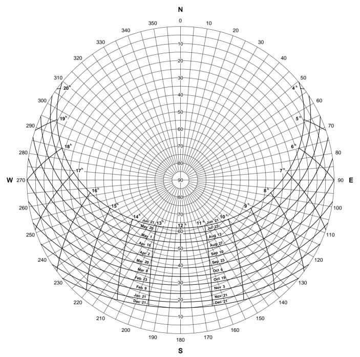
The diagram shows the altitude and azimuth of the Sun for a range of local apparent solar times from sunrise to sunset at latitude N  $51^{\circ} 30'$  (which is the latitude of London) for a series of dates throughout the year. A separate diagram for a specific latitude, which may be needed for better accuracy, will be supplied upon request.
