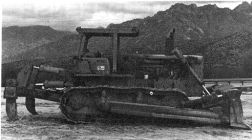
Bulldozer. Note the smoke stack (exhaust pipe).
