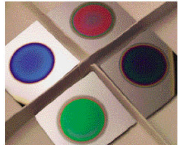
Fig. 3 This image shows four different types of porous silicon, where the pore size is varied. Thus, since pore size determines the luminescence spectrum the chips are different colors. (Courtesy Rochester University.)
