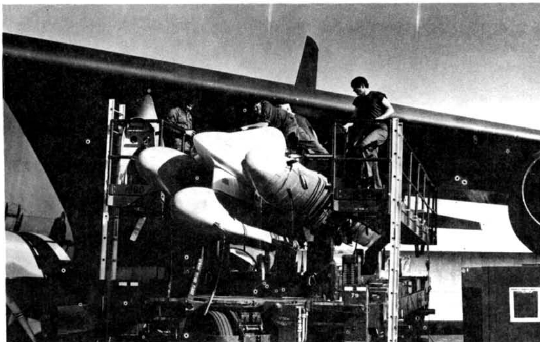
Members of the 7th Munitions Maintenance Squadron load an ALCM pylon onto a B-52H at Carswell AFB, TX, 10 December 1986
