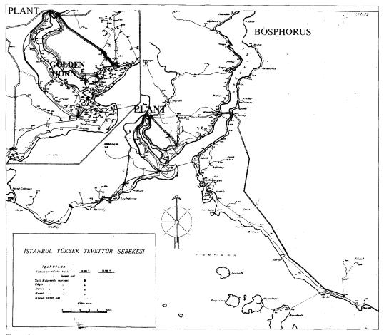
Figure 1 Power distribution network of the Plant
