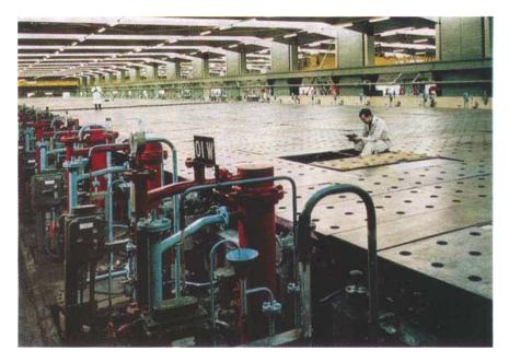
World production of chlorine by the electrolysis of brine is about 25 million tons a year. Some large estimates of platinum consumption as platinised-titanium anodes in this industry are now unlikely to be realised since the development of a ruthenium oxide coating on titanium
