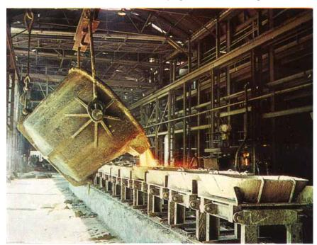
Flotation concentrates are smelted to a copper-nickel-iron matte. This is cast into moulds, broken up and sent to the refineries for extraction of copper, nickel and the six platinum metals
