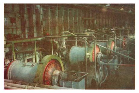
The ore is first crushed in a series of jaw crushers and is then fed to the primary and secondary ball mills
