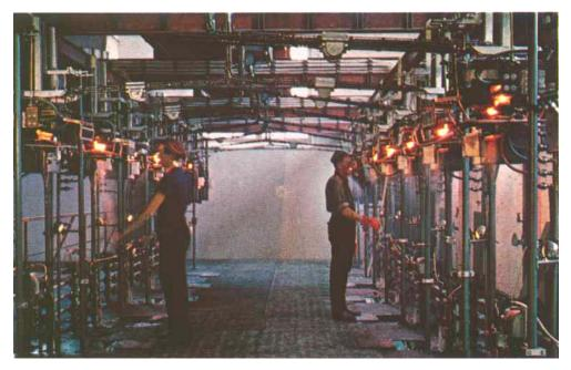
The manufacture of glass fibre involves the rapid flow of glass at around  $1,400^{\circ}C$  through a series of orifices which must retain their size and alignment. The electrically heated bushings are universally made in rhodium-platinum alloys
