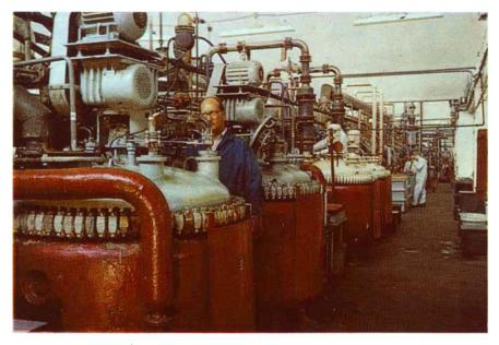
The initial stage in the Johnson Matthey wet process refinery involves digestion of the enriched concentrates with aqua regia to dissolve the platinum and palladium, leaving the iridium, rhodium, ruthenium and osmium as insoluble residues to be treated separately
