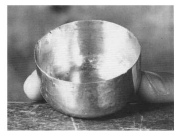
Iridium crucibles are now greatly in demand for the growing of oxide single crystals at temperatures around 2000°C but as long ago as 1908 a number of small crucibles were made in iridium by Johnson Matthey at the request of Sir William Crookes. One of these crucibles still survives in the company's possession
