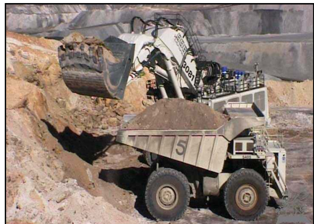
Shovel loading overburden onto a Dumper Truck
