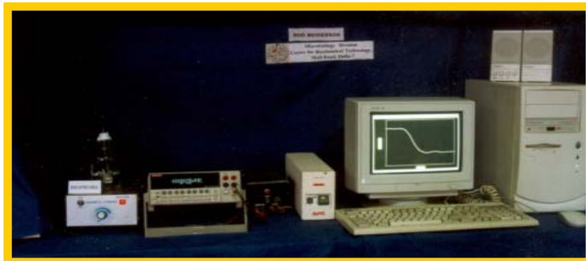
BOD BIOSENSOR Experimental Set up
