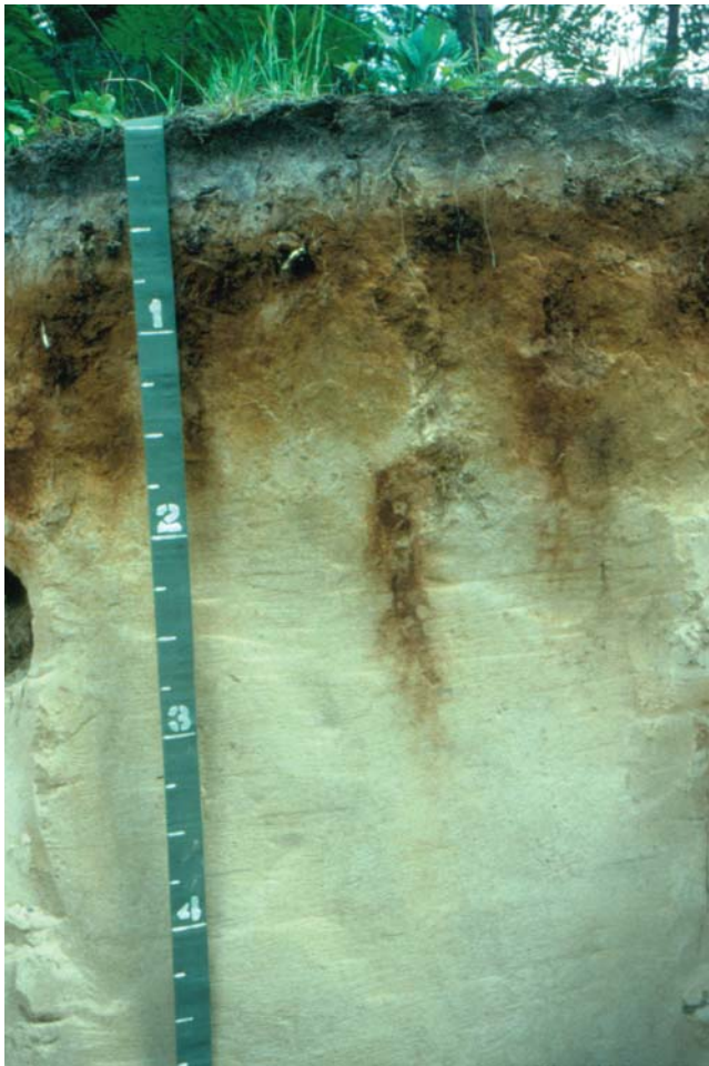
Figure 2.—Typical profile of Crowell fine sand, which formed in eolian deposits on dunes. Depth is marked in feet.
