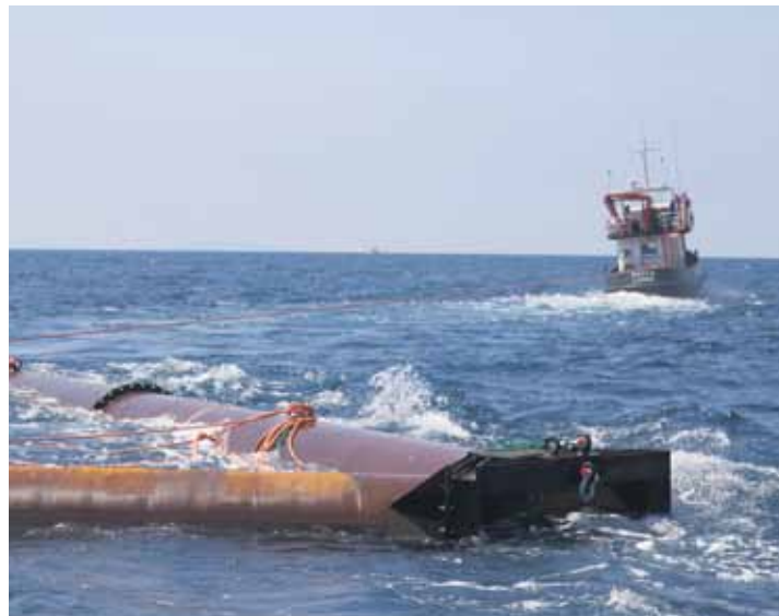
40South’s ‘hybrid’ wave power generator
