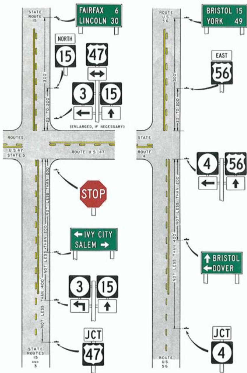
Figure 2-7b. Typical route markings at rural intersections (for one direction of travel only).
