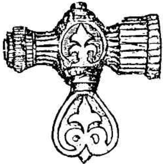
Original gas cock used on the ground floor chandeliers to turn on and off gas. The pipes supplying the gas are buried in the ceilings.
