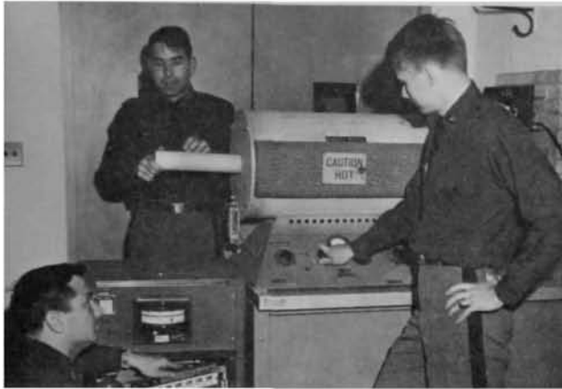
Diffusion furnace used to diffuse impurities into a semiconductor wafer.
