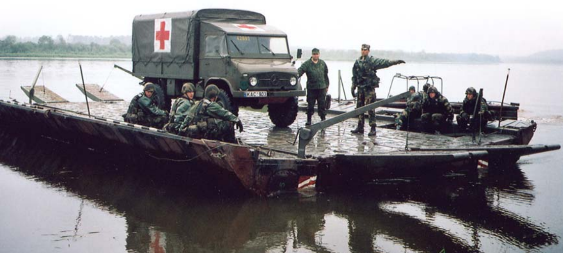
◀ A pontoon ferry built by military engineers transports military equipment
