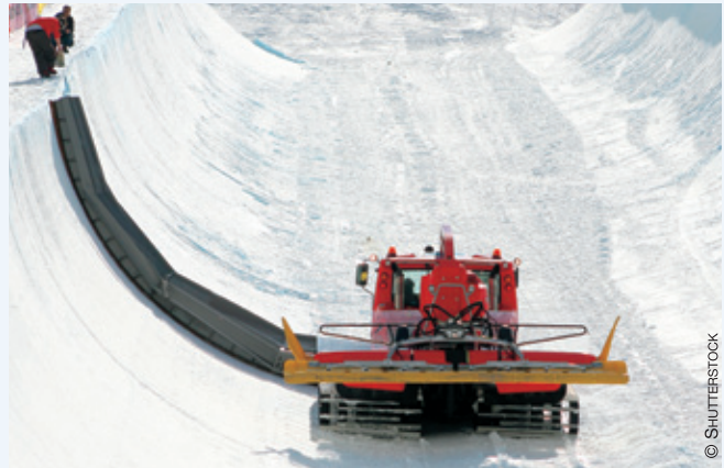
A snowcat fitted with a Pipe Dragon grooms a halfpipe in preparation for a competition.
