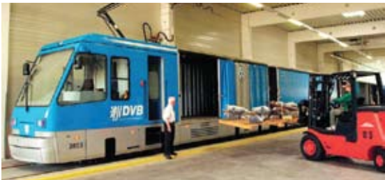
Possible transport solution for Bickerdike pier and the Technoparc. As the VW cargo tram shows, light rail systems can transport more than just passengers. Source: Gläserne Manufaktur
